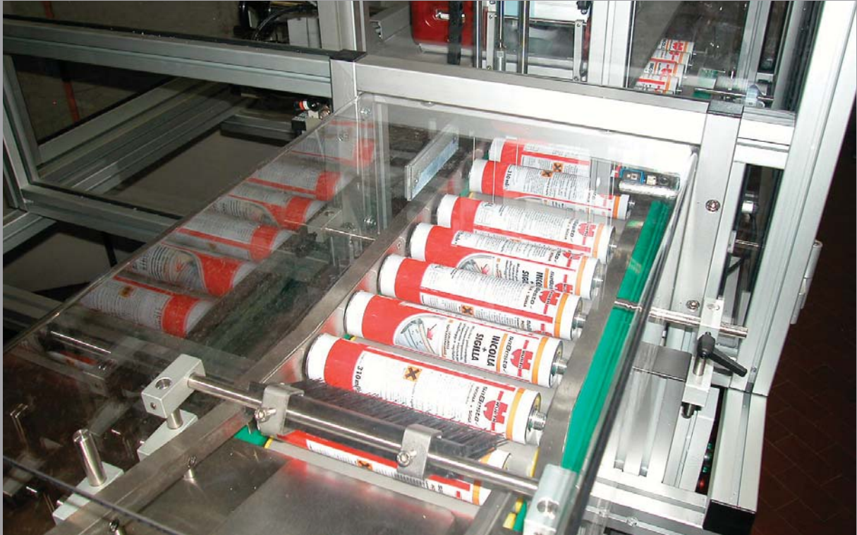
Wraparound labelling on laid cylindrical items
